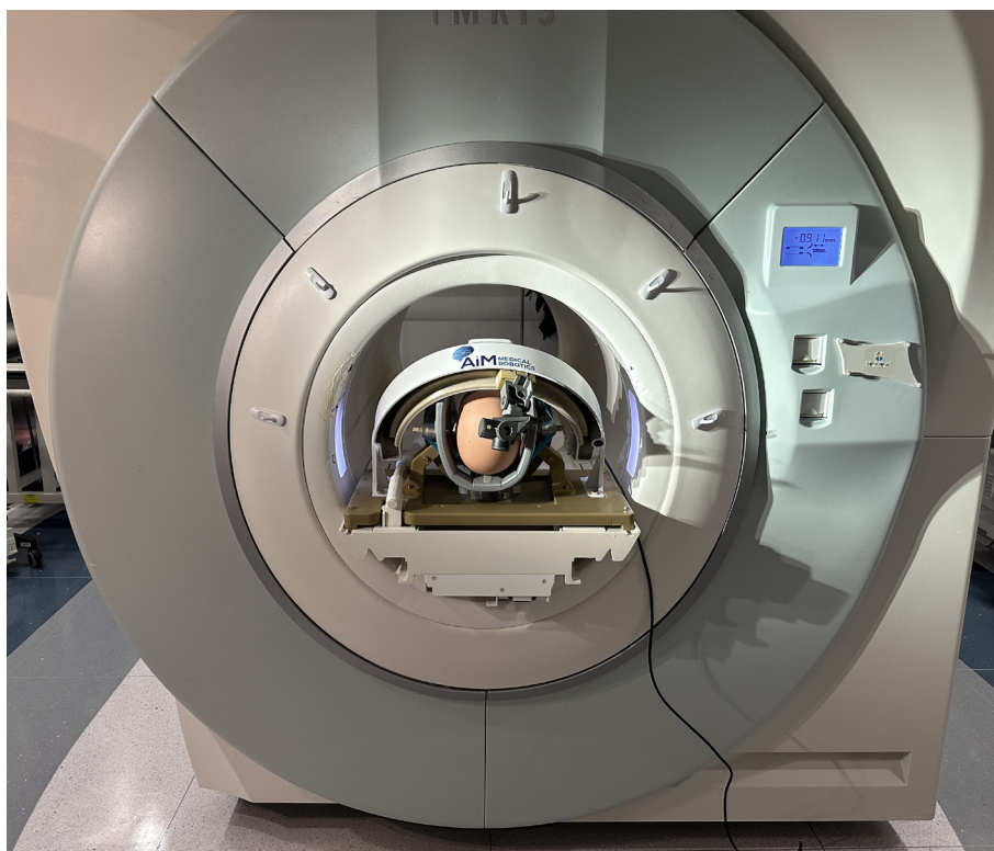
AiM's fully MRI-compatible robotic stereotactic frame (Source: AiM Medical Robotics)
